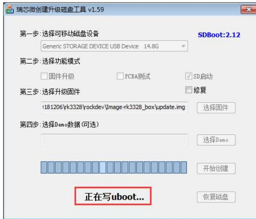
8) After burning, the display of SD\_Firmware\_Tool is as shown in the figure below. At this time, click the OK button to close SD\_Firmware\_Tool, and then you can unplug the TF card from the computer and insert it into the development board to start
